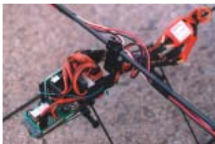
A close-up view of the micro-size radio gear that controls my aircraft.
